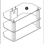
7. Place short legs onto panel and screw barrel nuts onto all threaded bars.
