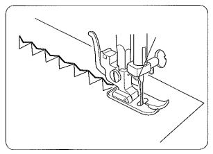
If forward and reverse feeds become unbalanced due to the type of fabric, adjust the balance by turning the stitch length dial as follows:
