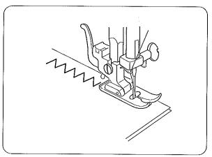
Simple zigzag stitching is widely used for overcasting, sewing on buttons etc.
