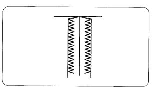
The zigzag stitch is used on the seam allowance to prevent fabric from fraying at raw edges.
