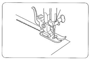
The stitch is sewn with two stitches forward and one stitch backward forming a seam that does not rip easily.
