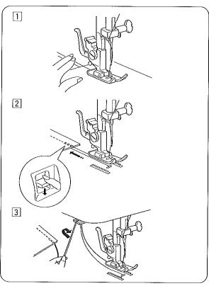
1 Raise the presser foot and position the fabric with its edge lining up with a seam guide line on the needle plate.
