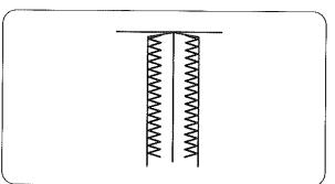
The zigzag stitch is used on the seam allowance to prevent fabric from fraying at raw edges.
