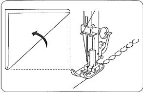
Place the folded edge along the slot of foot. The needle should fall off the edge of the fabric on the right forming a tuck.
