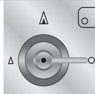
In models with safety valve, after ignition, the knob has to be held down for a few seconds to allow the thermocouple to heat up. The burner might go off when the knob is released: this means the thermocouple has not heated up sufficiently.
