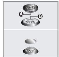
To work well, the ignition plugs and thermocouples must always be very clean. Check them frequently and clean them with a wet cloth if necessary. Any dry residue should be removed with a toothpick or a needle.
