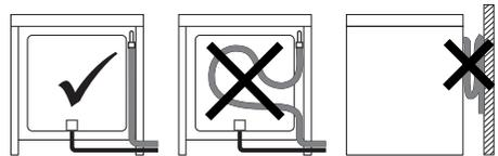
Make the connection to the gas mains using a rubber hose whose specifications comply with current standards (verify that the reference standard is stamped on the hose).
