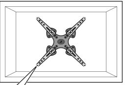
Holes do not line up and small adjustment is required before you fully tighten
