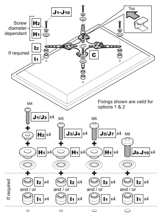
Attach the bracket to the back of your TV using suitable screw, reducer and spacer combinations.
