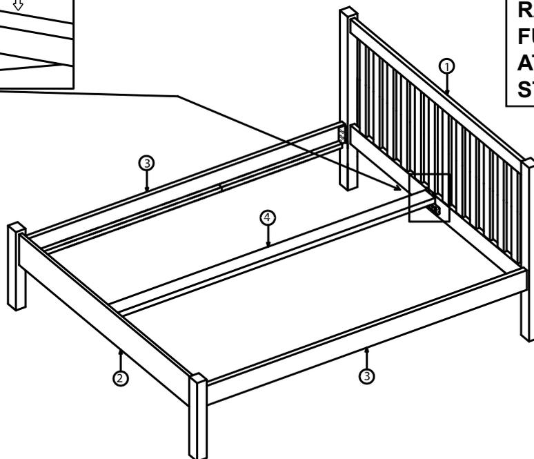
**AFTER INSERTING CENTRE RAIL, TIGHTEN ALL FIXINGS FULLY INCLUDING BOLTS AT SIDE RAILS (FROM STEPS ONE AND TWO)**
